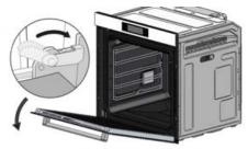
The hinge is normally inserted
